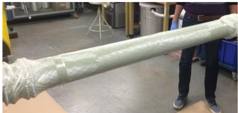
Figure 2: Small-scale turbine shaft that was fabricated to demonstrate the feasibility of a filament-wound design.
