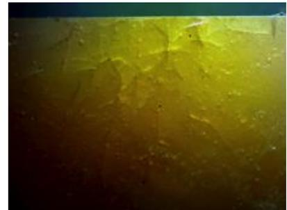
Photo of polymer matrix cracking on the backside of a sample tested under blunt, low-energy impact.
