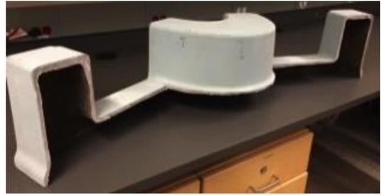
Example aquatic play part from Waterplay Solutions, using the modified coating material.
