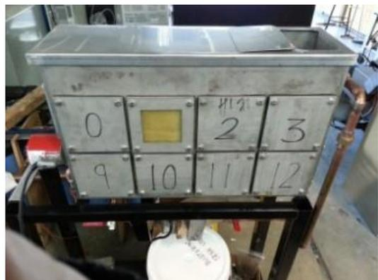
CRN blister tank for material exposure tests, simulating warm, flowing water in sewers.
