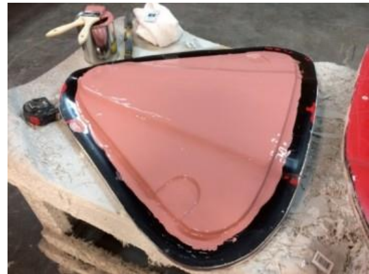
Mould with polymeric storage film brushed on prior to storage outdoors.
