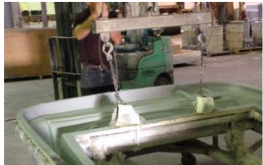
Boat deck being de-moulded after curing.
