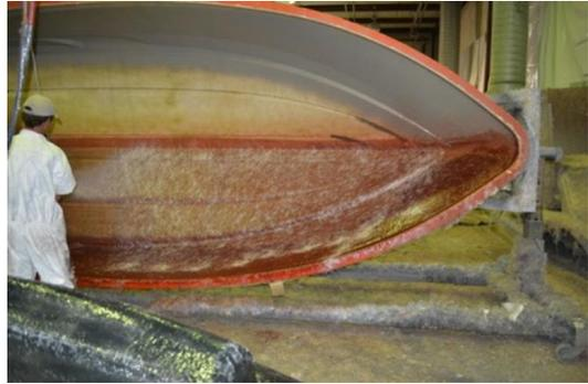
Bulk laminate is sprayed onto a boat hull and left to cure.
