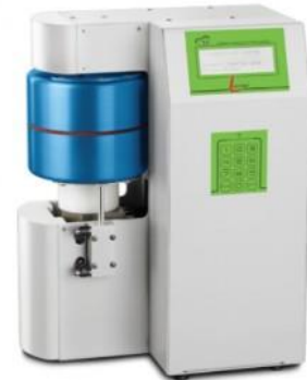
FOX50 thermal conductivity tester.
